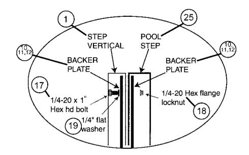
The above illustration shows correct hardware placement when installing backer plates. Refer to exploded view for backer plate locations.
