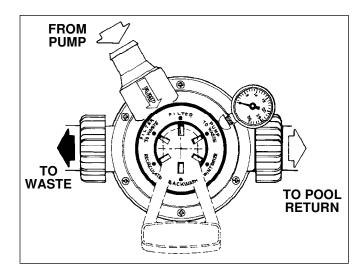
through the valve on top of the filter bypassing internal filter components and travels back to the pool at a rapid rate
