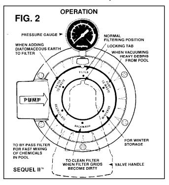
filter will vary with pool size, pool use, amount of airborne dirt and debris, and the chemical treatment you give the water. Backwashing should be done when the Sequel II<sup>™</sup> pressure gauge reads 5 to 7 pounds higher than initial start-up pressure. Example: If the pressure guage reads 10 pounds at the start of a clean filter, you should backwash when the gauge reads from 15 to 17 pounds.
